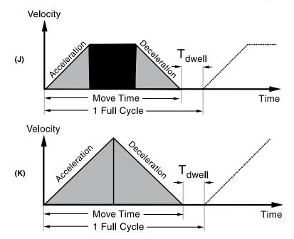
If using a trapezoidal (J) or triangular (K) move profile, the following is needed...
