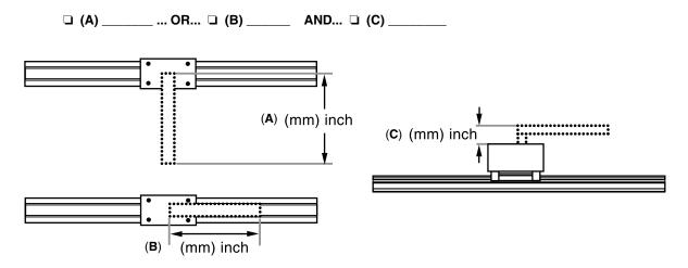
3) **Rail Mount Orientation?** The force needed to move the load is dependent on the orientation of the load relative to the force of gravity. For example, total required force in the horizontal plane (D) is a function of friction and the force needed for load acceleration ( $F_f + F_a$ ). Total force in the vertical plane is a function of friction, load acceleration, and gravity ( $F_f + F_a + F_a$ ).
