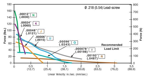
NOTE: All chopper drive curves were created with a 5 volt motor and a 40 volt power supply.
