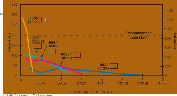
NOTE: All chopper drive curves were created with a 5 volt motor and a 75 volt power supply.
