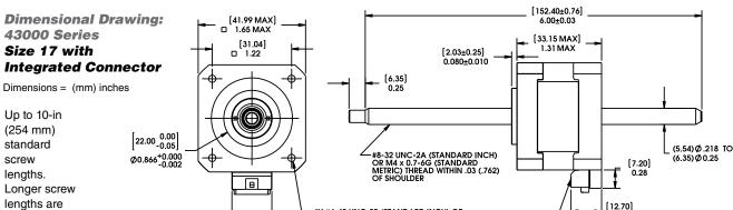
4X #4-40 UNC-2B (STANDARD INCH) OR 4X M3 x 0.5-6g (STANDARD METRIC) THREAD X 0.15 (3.8) DEEP
