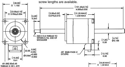
**Motor Connector:** JST part # S06B-PASK-2 **Mating Connector:** JST part # PAP-06V-S
