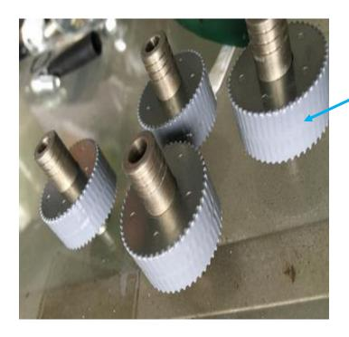
The gray epoxy material added and cured on the motor rotor just prior to turning operation
