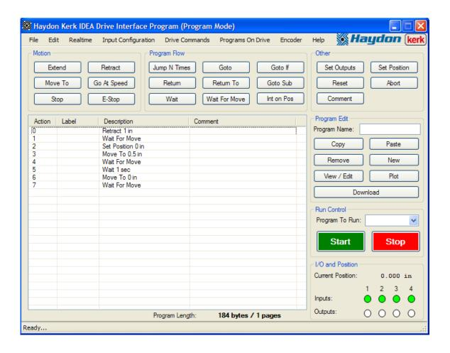
**Example Five:** In this example, we will first find the fully retracted position of the motor within a linear application, then the motor will move to the 0" position if input 1 is high and input 2 is low, move to the 1" position if input 1 is low and input 2 is high, or stop if inputs 1 and 2 are both high, or both low.
