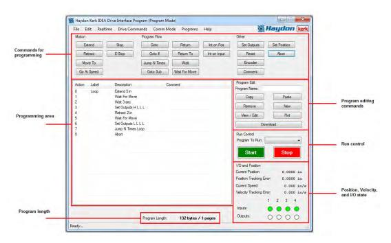
The I/O and position section provides constant feedback from the drive pertaining to the current state of the drive. This area can also be used to control the state of the outputs, as well as the inputs if in simulation mode.
