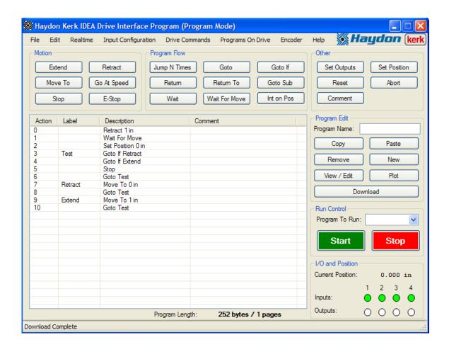
**Example Six:** In this example, we will first find the fully retracted position of the motor within a linear application. The motor will continuously move in the extend direction, until getting 0.9" from the fully retracted position. When the 0.9" position is reached, the motor will retract back to the 0" position, and resume the extend. If at any time during the program, input 1 changes state, the program will abort.
