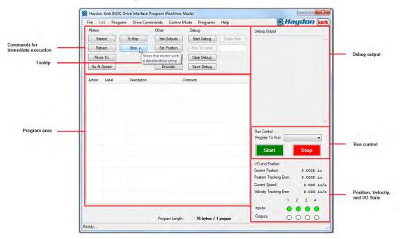
In the Realtime mode, each command executed from the "Commands for immediate execution" section elicits an immediate action from the drive.
