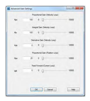
This window will allow users to adjust the PID control loop of the brushless IDEA drive. Users can adjust the proportional, integral, and derivative gains of the velocity loop, as well as the proportional gain of the position loop and the feed forward of the current loop. Users should only adjust these gains if they are familiar with their functionality. Future software revisions will expand on the Help function within this form to aid users in fine adjustments of the control loop.
