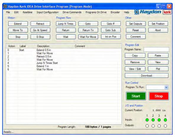
**Example Three:** This example will extend the motor within a linear application .5", turn all four outputs high, wait .5 seconds, turn all outputs low, retract the motor .5", turn all four outputs high, wait .5 seconds, turn all outputs low, then end the program. We will accomplish this by using a subroutine.
