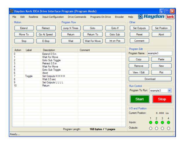
**Example Four:** This example is different in that the motor within a linear application does not need to start in the fully retracted position. We will perform a homing routine, to find the fully retracted position, and then move to 0.5" from that point, wait 1 second, and then return to the fully retracted position.
