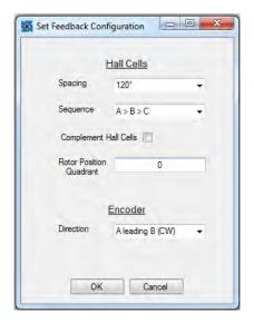
The drive is capable of driving a motor with 60° or 120° hall cell spacing.
