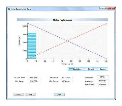
In addition, this graph will also display the motor limitations set by the software. Software limitations are designed with the intention to allow the user to drive the motor at its peak efficiency. Generally, a brushless motors' peak efficiency point falls between 15- 30% of the rated torque and slopes down beyond that. This is also within the area where a motor can operate continuously and is ideal for maximum motor life.
